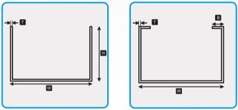
T = Thickness B = Bend H = Height W = Width
